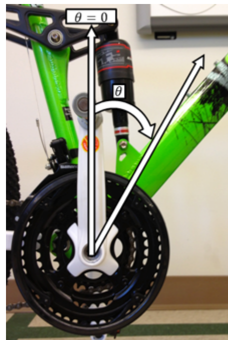
Figure 4: \theta = 0 is the orientation when the crank arm is directly vertical with the pedal bar above the crank bolt.
