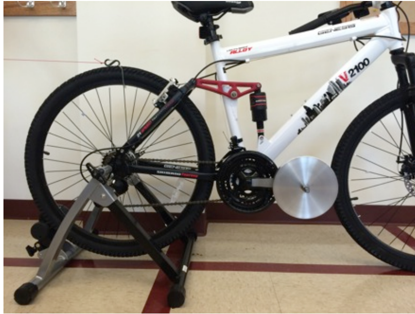
Figure 2: The essential static setup. The crank arm is horizontal and holds disk masses on the pedal bar. The rear wheel is held stationary. A carabiner is attached to a zip tie that is zipped around the rear wheel, directly above the rear axle. The carabiner is attached to a string that is pulled horizontally to the left. The other (unseen) side of the string is attached to a force sensor. The force sensor measures the tension in the string.
