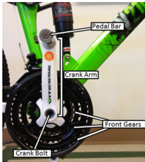
Figure 1: The front part of the drive train of our bicycle. Applying an appropriate force to the pedal bar causes it, the crank arm, and the front gears to rotate. All of these components together will be referred to as the crankset .
