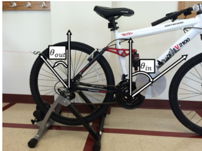
Figure 5: A 1-kg mass is attached to the pedal bar which is at an angle of \theta_{in} = 50^\circ . The carabiner is attached to the zip tie such that \theta_{out} = 30^\circ . The string is pulling horizontally to the left. The string is attached to a force sensor. The chain is passing over the front gear of largest diameter and the rear gear of largest diameter.
