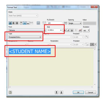
Step 12: Using the properties of the Model. Be sure to set your dialog box like the one below. One important step that must be done is to select the marked box below after selecting the type and property choices. Then select ok.
