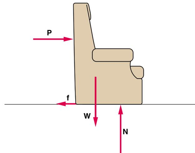
**Figure 4.15** Four forces act on a chair being pushed across the floor, the weight  $\mathbf{W}$ , the normal force  $\mathbf{N}$ , the force  $\mathbf{P}$  exerted by the person pushing, and the frictional force  $\mathbf{f}$ .
