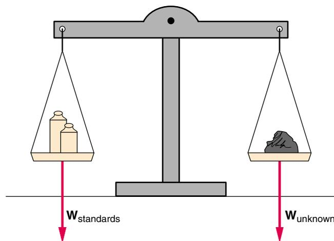
**Figure 4.8** Comparing an unknown mass to standard masses on a balance.
