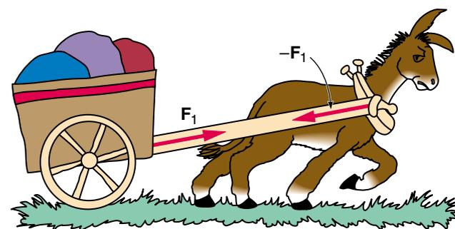
**Figure 4.13** A mule and a cart. Does Newton’s third law prevent the mule from moving the cart?
